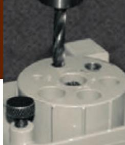
General's Pro Doweling Jig is a precision jig that assures the accurate line-up of dowel holes in furniture and carpentry. Simply clamp the jig onto
