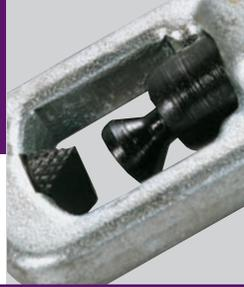
Telescoping Gages are used for quick and accurate measurements of inside diameters of holes and widths of slots from which micrometer measure-
