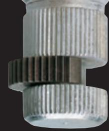
Internal Pipe Wrenches are used for the removal of broken thread ends of pipe, pipe plugs and fittings lodged inside other pipes.
