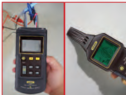
Tracing a cable behind a wall
