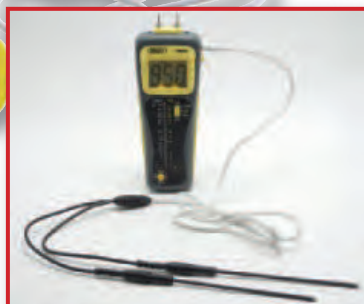
The MMD900 with the optional MP905 Deep Wall Moisture Probe
