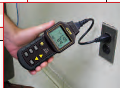
The short test cable improves voltage-drop measurement accuracy
