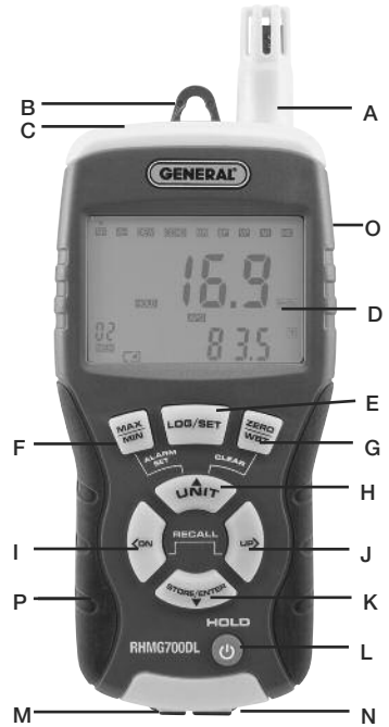
Fig. 1. The controls and physical structures of the RHMG700DL
