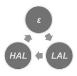
Also remember that when  $\varepsilon$ , LAL or HAL is flashing, you have only 30 seconds to change its value or setting by pressing the  $\clubsuit$  LOG button or the °F/°C  $\clubsuit$  button. Thirty seconds after the last button push, the IRT659K's Auto Power Off function will activate and shut down the unit.
