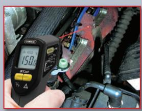
With a 600°F measurement ceiling, the unit can handle any automotive application
