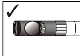
Remove the blue circular protective film from the mirror by pulling on its tab with a tweezers.
