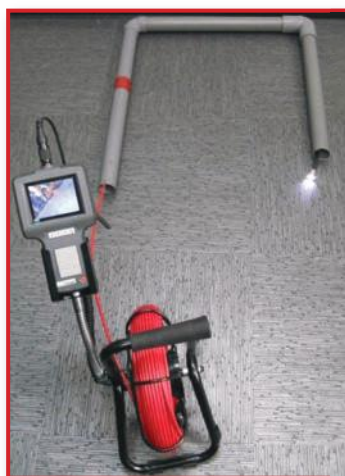
The DPS16/P16PIP probe is flexible enough to make two 90° bends in a 1.6 in. (40mm) diameter pipe
